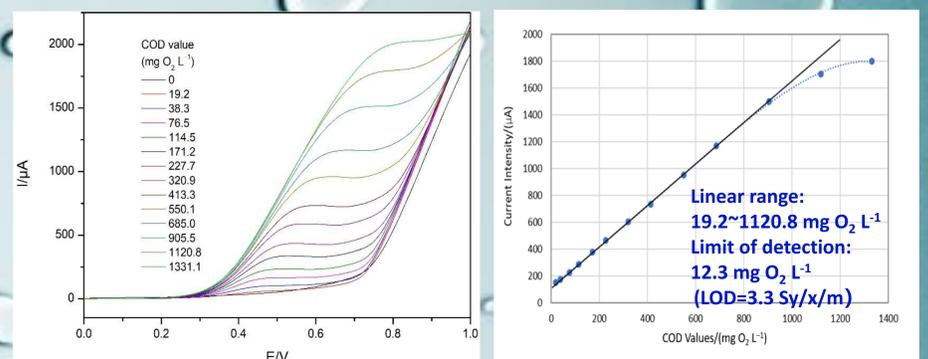
Figure 4. (A) Oxidation curves of cyclic voltammetric responses of electrode E1 with the increase of addition of glucose in 0.05 M NaOH solution. (B) Calibration plot of intensity of current at  $E=0.7050$  of electrode E1 as a function of COD values (glucose as standard substance). Potential scan window,  $-1.0$  to  $+0.7$  V vs. Ag/AgCl (3.0 M KCl). Scan rate, 50 mV/s.
